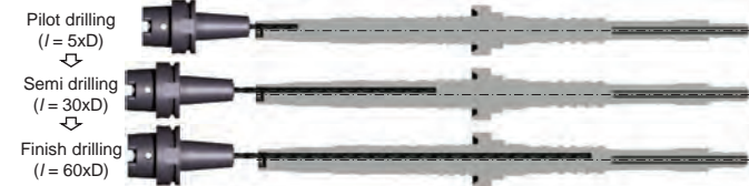
Three-stage deep hole drilling process
